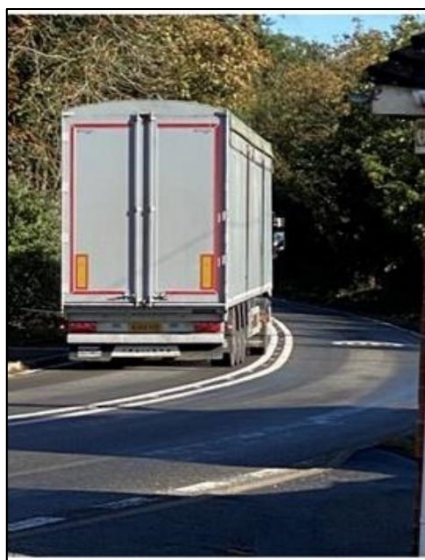
Plates 4 and 5: Standard width and length HGVs sit just within double white line system at Little Glemham
